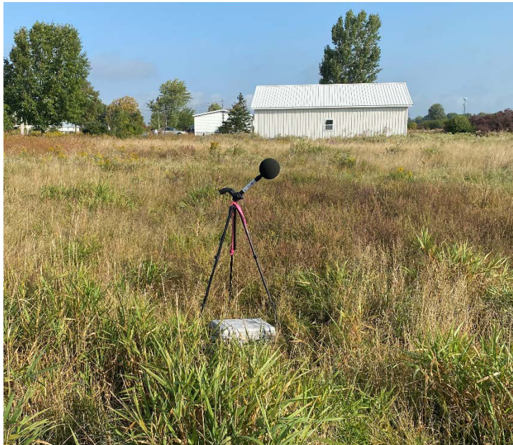
Figure 1-2 Location 1 -- Sound Level Meter
