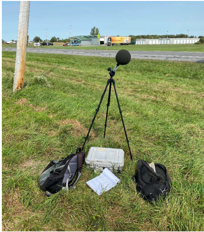
Figure 1-3 Location 2 - Sound Level Meter
