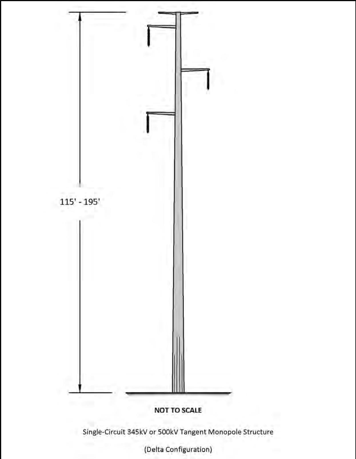
Figure G-14. Single-circuit 345-kV or 500-kV tangent monopole structure (delta configuration).
