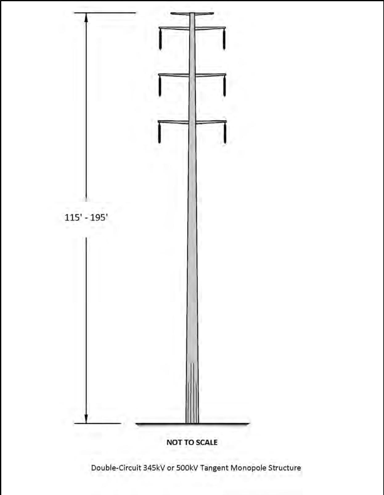
Figure G-16. Double-circuit 345-kV or 500-kV tangent monopole structure.
