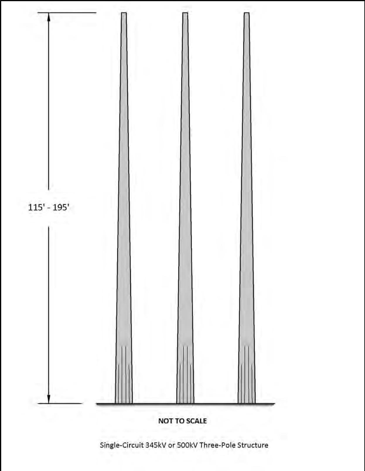
Figure G-20. Single-Circuit 345-kV or 500-kV three-pole structure.
