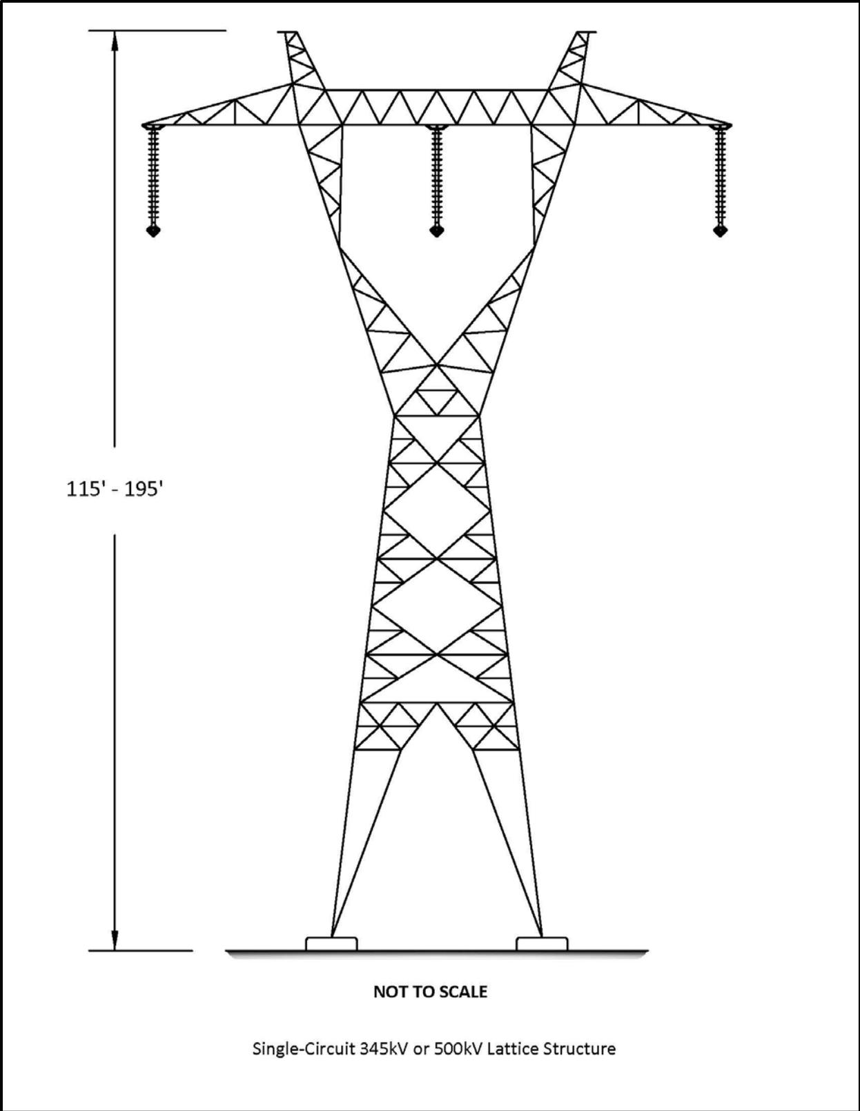
Figure G-13. Single-circuit 345-kV or 500-kV lattice structure.
