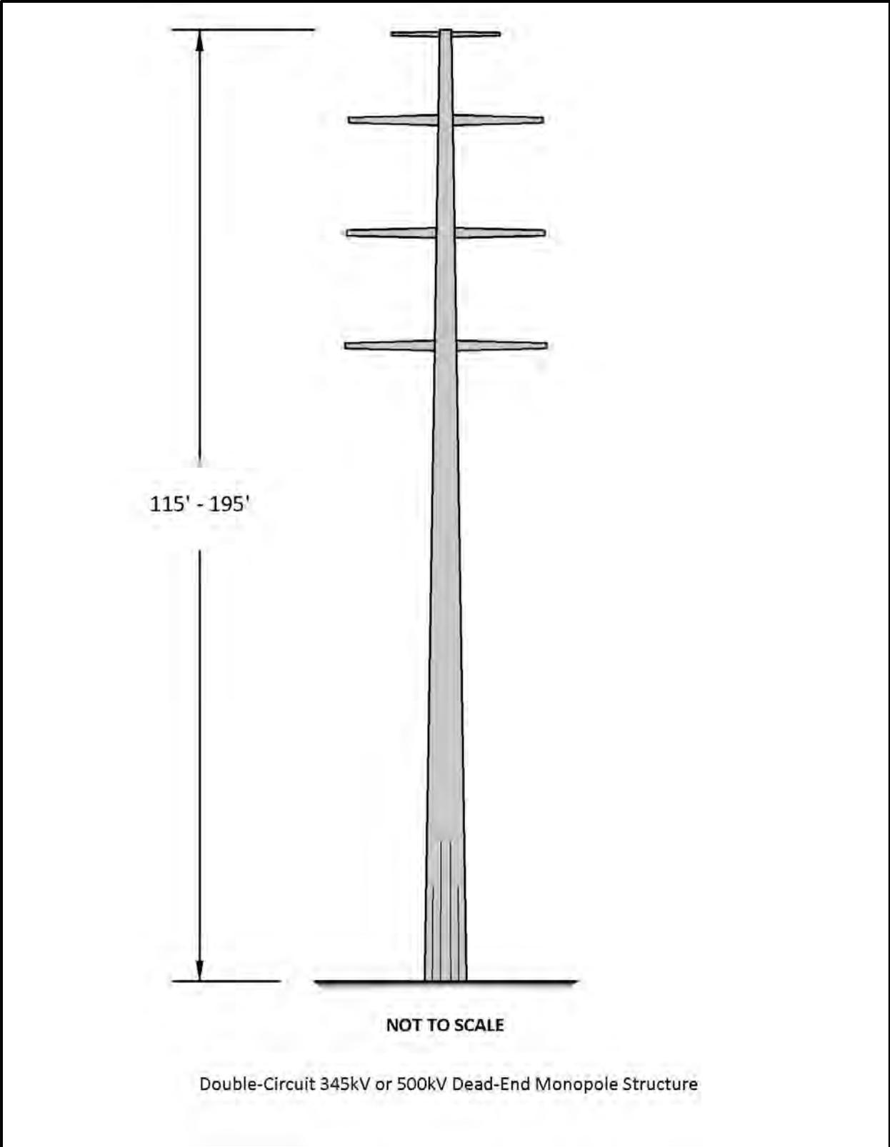
Figure G-18. Double-Circuit 345-kV or 500-kV dead-end monopole structure.
