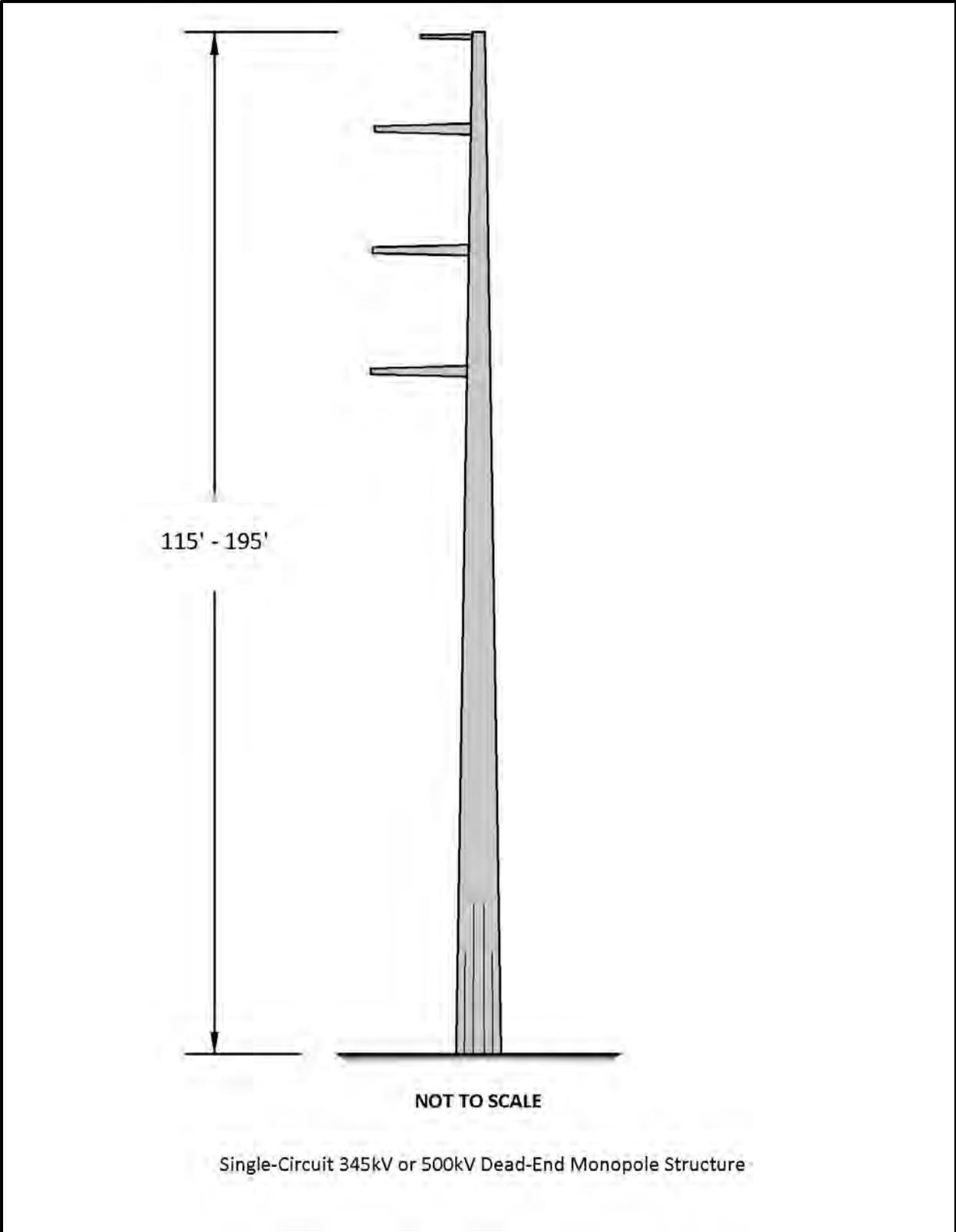
Figure G-17. Single-Circuit 345-kV or 500-kV dead-end monopole structure.
