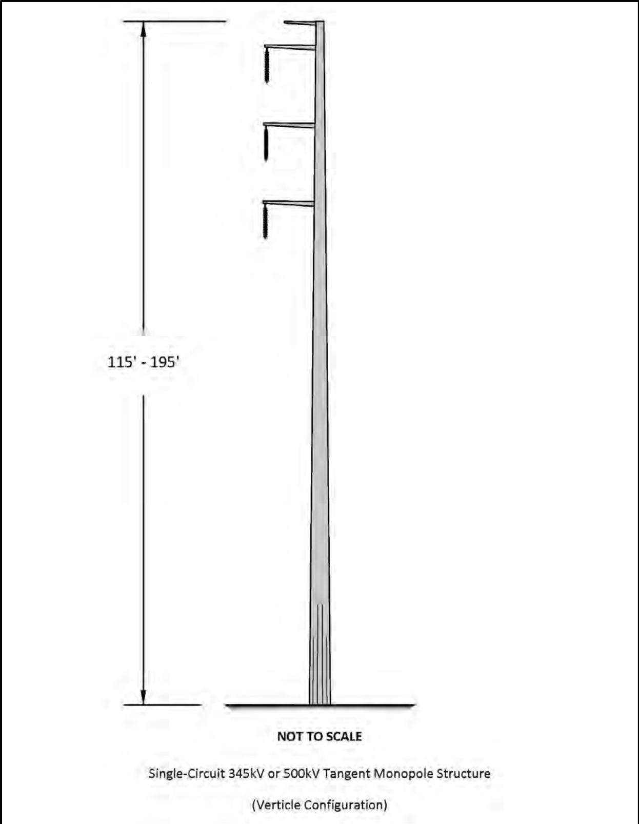
Figure G-15. Single-circuit 345-kV or 500-kV tangent monopole structure (vertical configuration).
